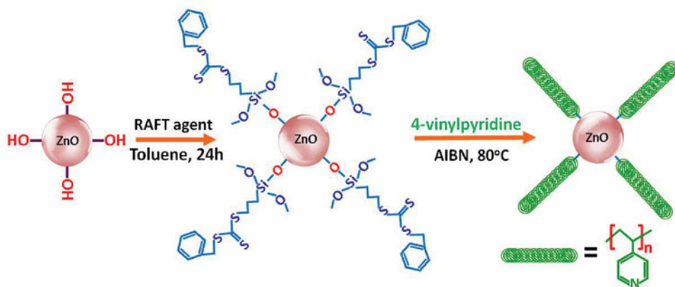
Scheme 1. A schematic representation for the synthesis of PVP-g-ZnO nanocomposites by RAFT polymerization technique.
